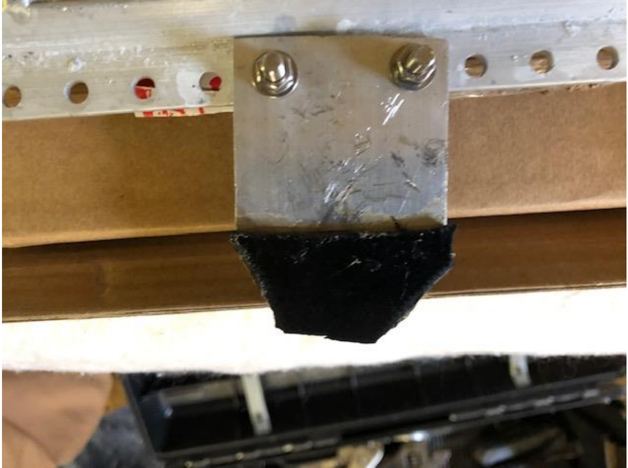
RUBBER ISOLATORS GLUED TO BRACKET TO ISOLATE FROM BODY MOUNT
