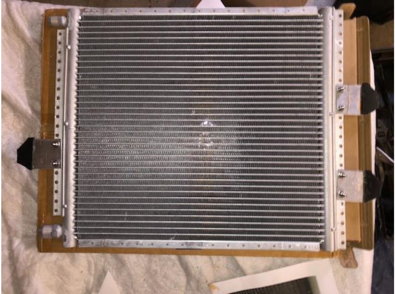
BRACKETS ATTACHED TO CONDENSER
