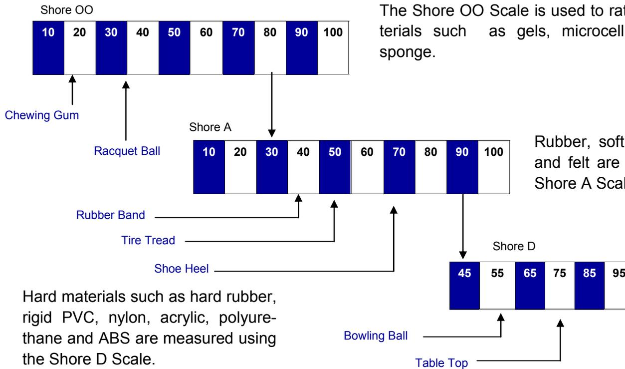
**Durometer is the International Standard for measuring the hardness of rubber, sponge, plastic and other non-metallic materials.**
