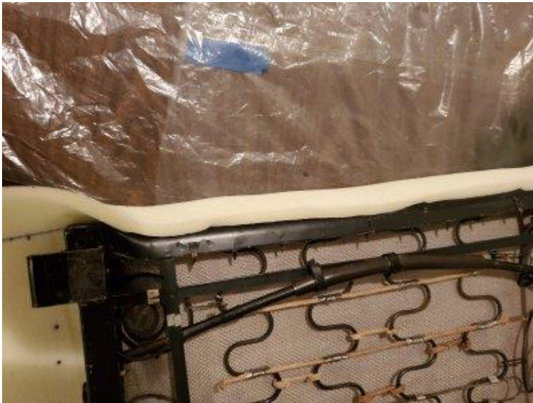
near the back, on the side glue directly to frame.
