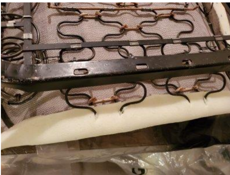
Done with first layer. Firm foam wraps around and is glued back onto itself - glue penetrates the burlap.
