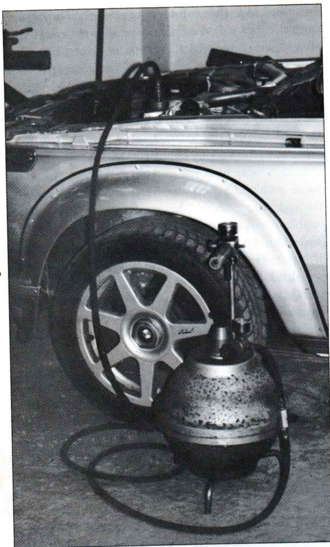
Pressure brake bleeding, using ATE equipment.
