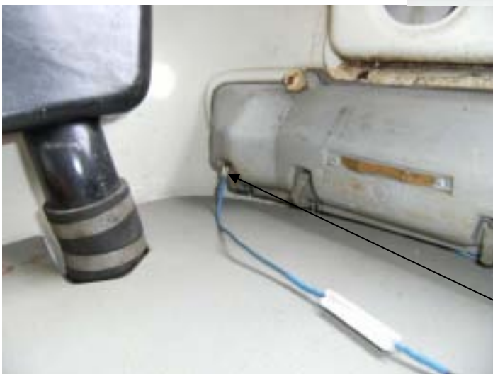
Doubler connection for the wiring loom and the resistor circuit.
