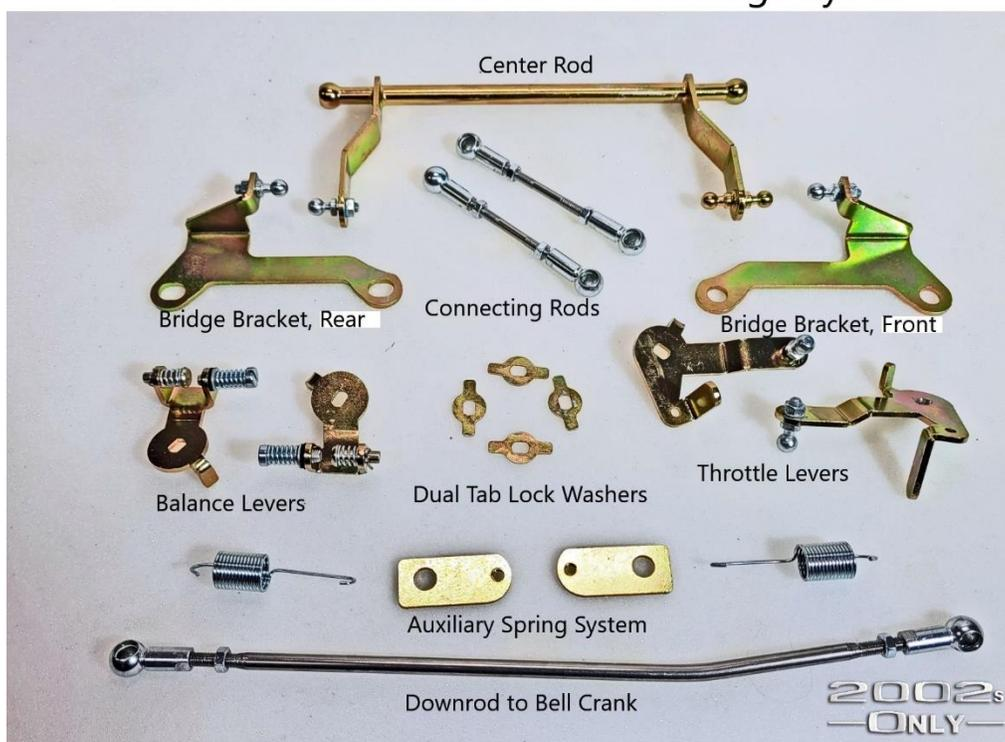
1. The Center Rod has one lever with one ball and one lever with two. The lever with two balls is positioned to the front of the engine.
