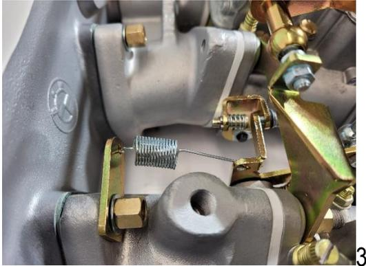
5. The Bell Crank Down Rod should be attached to the bell crank first. With the butterflies completely closed and synchronization complete, the Down Rod adjustment nuts are then used to match the Center Rod linkage lever to the Down Rod.
