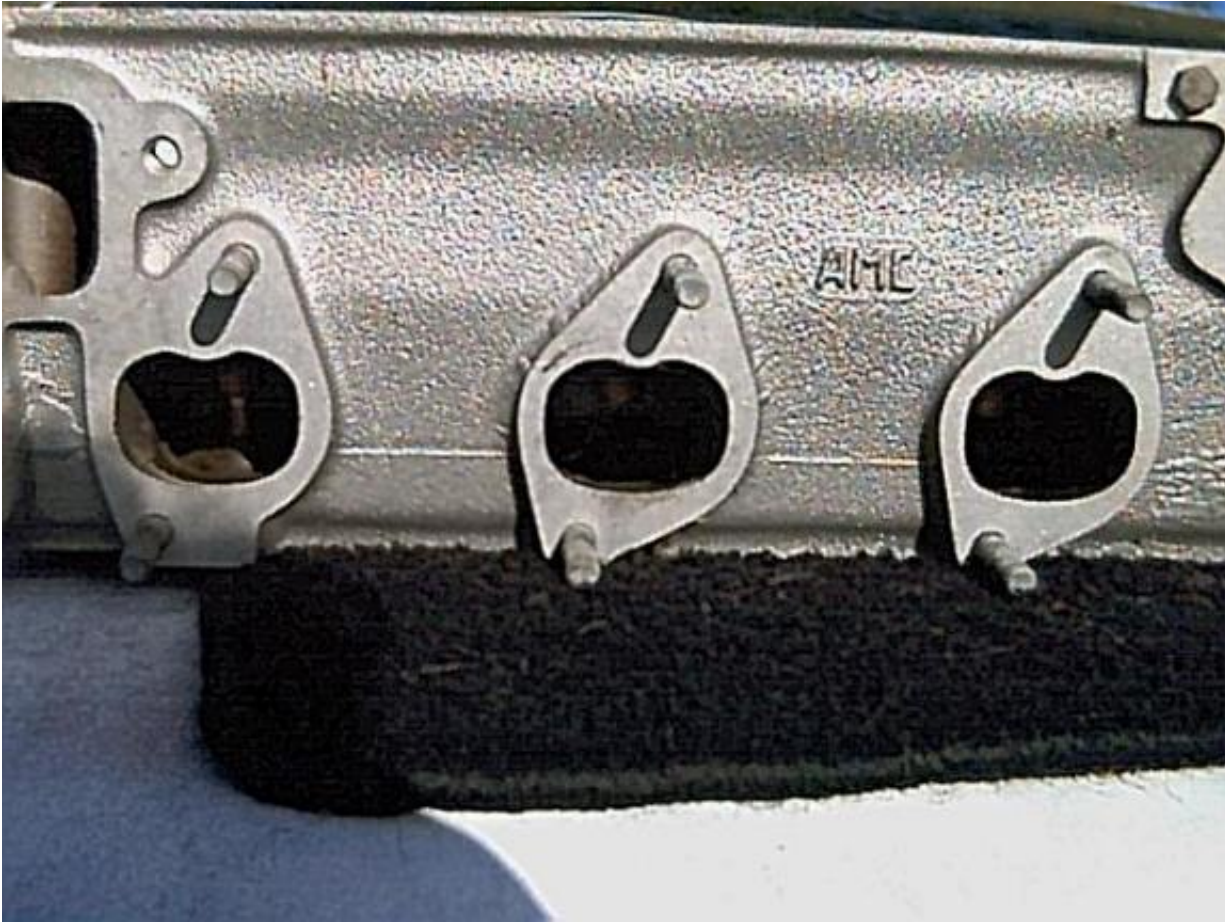
AMC head showing casting mark - Mike Wassall
