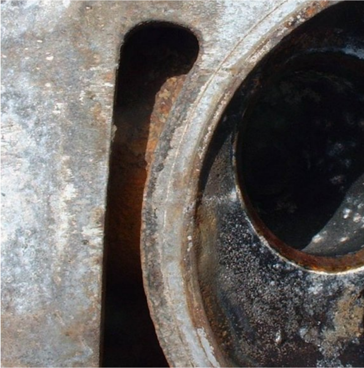
Crack between combustion and chamber and coolant passage on 1977 head Crack is in center of picture (faint white line) - Peter Florance
