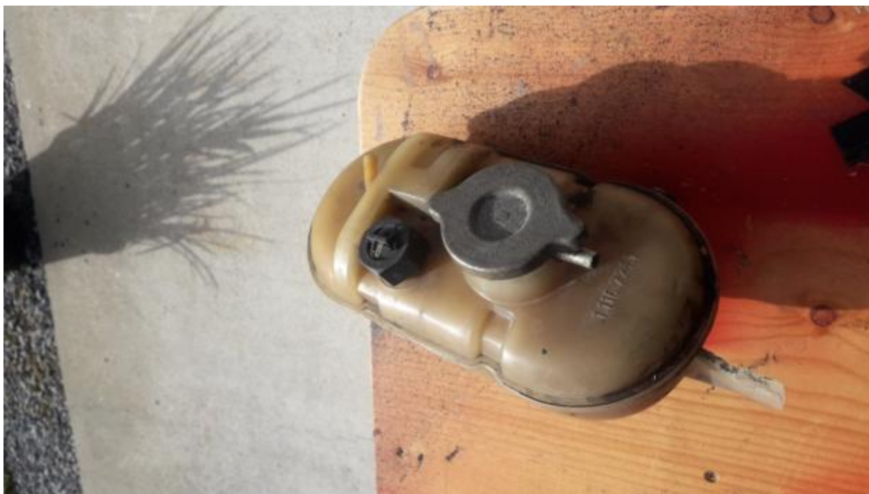
Header tank in working condition no leaks
