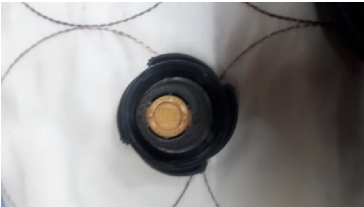
Pressure cap in good condition
